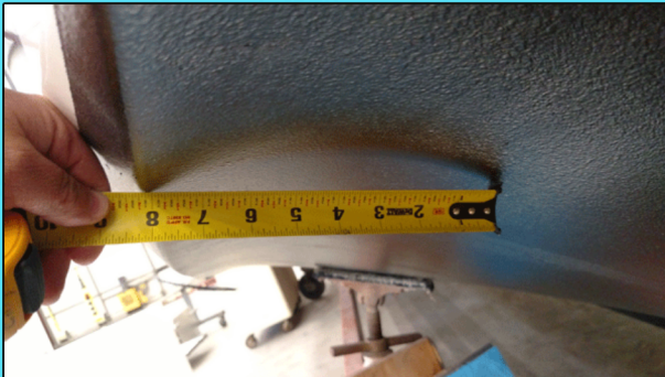
6.5 feet back from bow 8 inch filled in to 0.75 inch curved air gap
