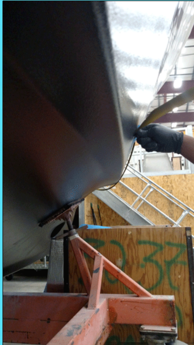
Aft End of the modified chine 13 feet from the bow
