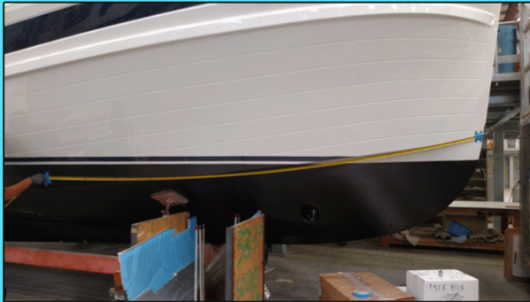
Area where chine has been filled
